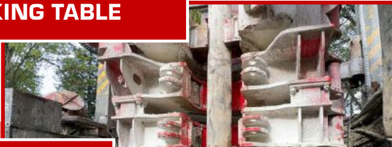
CAN BE USED AS A CASING EXTRACTOR
