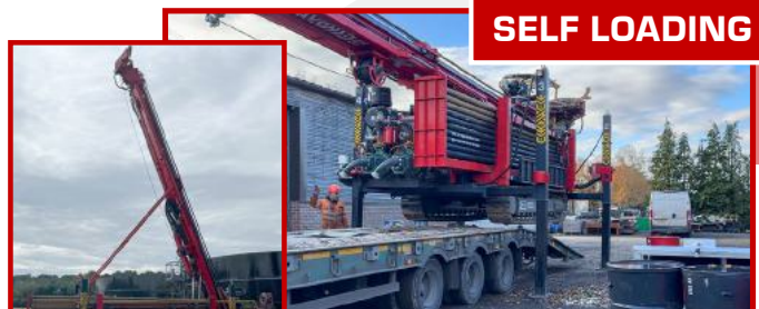
4 x HYDRAULIC LEGS TO LIFT & LEVEL THE RIG
