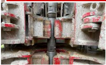
TRIPLE CLAMPS 1 ROTATING & 2 FIXED 12 1/2" (320 mm) OPENING
